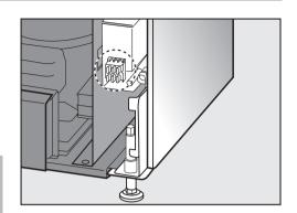
Choose the desired switching contact and connect according to alarm system requirements.
